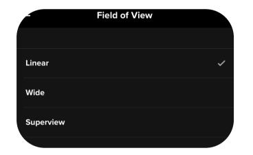
Field of View: Linear (otherwise it looks distorted/fisheye) Make sure 'Video Stabilization' is toggled on
